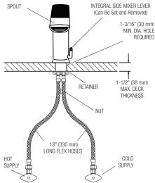
When the BASYS Series faucet is installed on a sink that has three (3) hole punchings, a Base Plate should be used. **Base Plates should be specified at time of order.**
