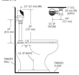
The Model 8115 valve is designed for installations where the water supply is roughed-in 24" (610 mm) above the top of the water closet.
