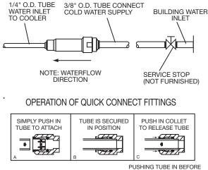
PULLING IT OUT HELPS TO RELEASE TUBE Open space rough-in design permits new installation or replacement of existing fountains and coolers with this Elkay cooler when rough-in is within the outline shown.
