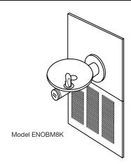
opens to allow water flow. No physical contact with cooler is required. A built in time delay is provided to prevent actuation by persons moving past cooler. There is a maximum running time of 30 seconds to prevent malicious damage to the cooler or water damage if sensor vision is blocked. Unit automatically resets when blockage is removed. Sensor range is adjustable.
