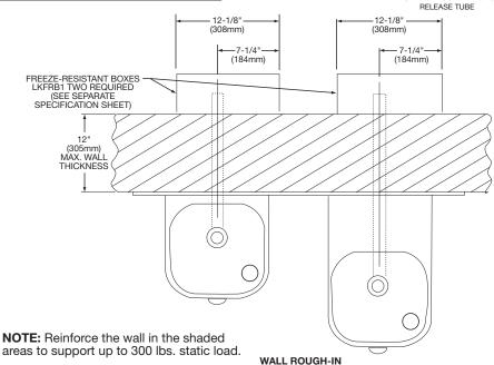
**WARNING:** The freeze-resistant box must be installed on an interior heated wall where the temperature does not drop below 50°F (10°C). The front of the box must have unobstructed air flow. Failure to maintain the interior wall temperature and the inside of the freeze-resistant box above 50°F (10°C) can result in damage to the box which could result in unrestricted water flow.
