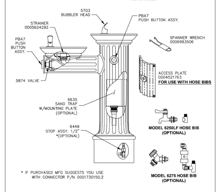
IMPORTANT: IF EITHER HOSE BIB IS USED IT MUST BE USED WITH SAND TRAP 6611. CANNOT OFFER HOSE BIBS AS AN OPTION WITH SAND TRAP 6635. IF A HOSE BIB IS PURCHASED, ACCESS PLATE 0004521763 MUST BE USED.
