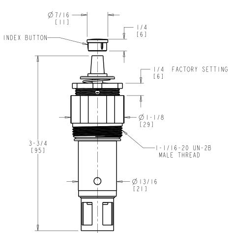
DIMENSIONS ARE IN INCHES AND [MILLIMETERS].
