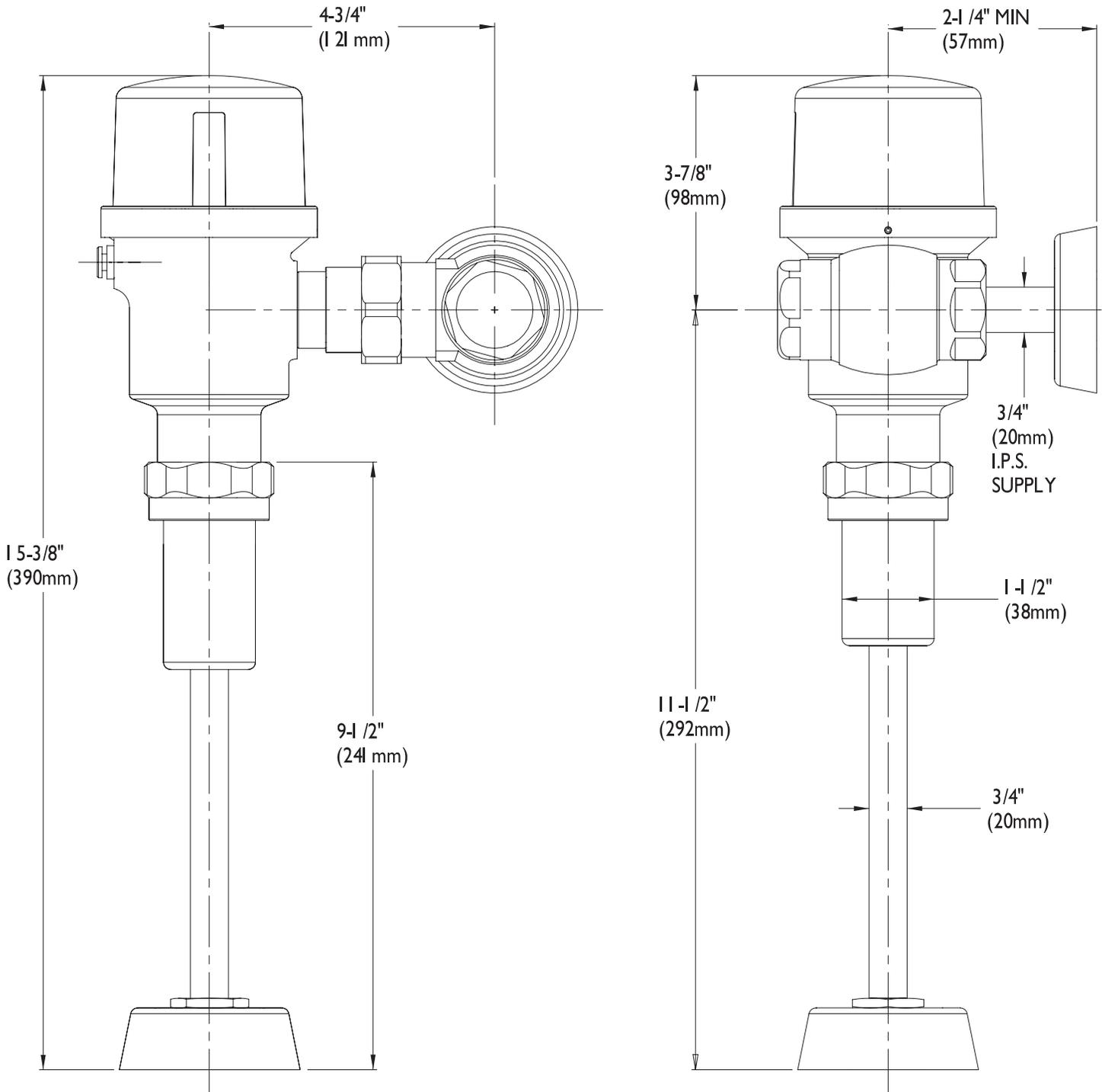
NOTE: All dimensions are in inches (millimeters) unless otherwise specified and are subject to change without notice. Unless otherwise specified, inlet is 3/4" NPT or 3/4" copper female and outlet is 3/4" NPSM female.
