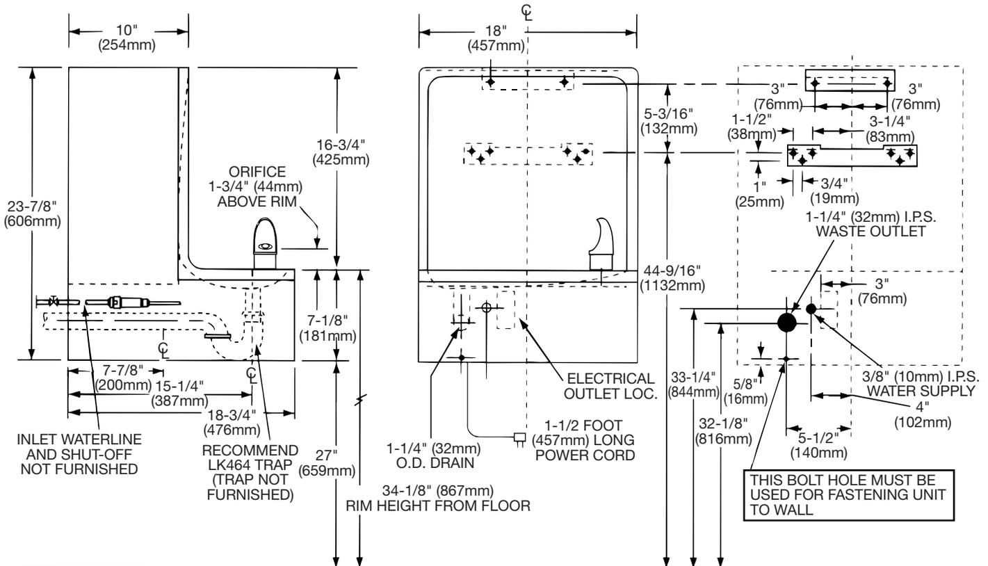
NOTE: INSURE PROPER VENTILATION BY MAINTAINING 6" (152mm) CLEARANCE FROM CABINET LOUVERS TO WALL ON EACH SIDE OF COOLER
