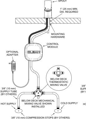
EFX Faucet with Below Deck Thermostatic for Hot and Cold Water Supply (shown with 4" Trim Plate)
