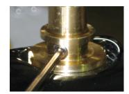
Remove the MV Stem assembly.Careful not to lose the inner stem.
