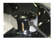
3. Remove the small Set Screw from the MV Handle Stem and place aside.
