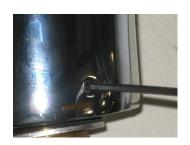
6. Pull the Faucet Body from the brass base. Care must be taken not to scratch or damage the brass base.
