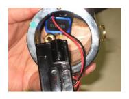
10. Remove the Battery Connector Cap and Battery Connector. Replace the old battery for the new one, and reconnect everything again.
