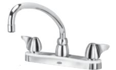
Polished chrome-plated 8" [203mm] brass deck faucet with a 9-1/2" [241mm] tubular brass swing spout and quarter turn ceramic disc cartridges. Unit is furnished with a 2.2 GPM [8.3 L] pressure compensating aerator (complying with ANSI A112.18.1 Standard for flow), 2" [51mm] vandal-resistant color-coded metal dome lever handles, mounting hardware and 1/2" NPSM coupling nuts for standard lavatory risers.
