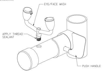
4. Apply a thread sealant and attach shower head to 1" nipple on upper shower arm. Fasten lever handle with screw located in extension. Secure pull rod to lever handle.
