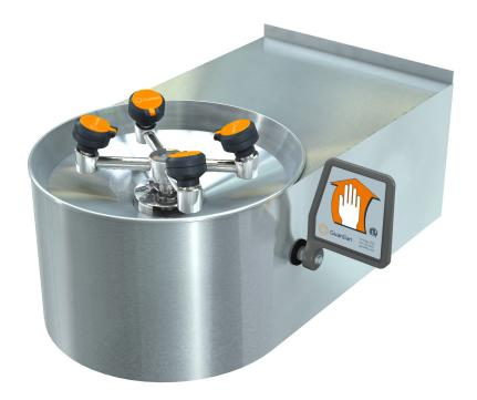
**APPLICATION:** Handicapped accessible WideArea<sup>™</sup> eye/face wash for wall mounting. Bowl is lowered and extended to permit access by wheelchair user. Profile of unit is "flattened" to comply with maximum height and knee clearance requirements. Unit has stainless steel bowl and wrap around skirt to conceal valve, drain and piping.
