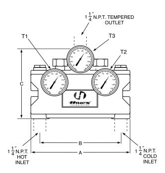
**Caution:** When maintaining and adjusting the mixing valve, the delivered flushing fluid temperature shall be 60°F (15°C) to 95°F (35°C). In circumstances where chemical reaction is accelerated by flushing fluid temperature, a medical advisor should be consulted for the optimum temperature for each application.
