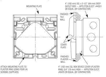
To ensure a perfect rough-in, Sloan recommends the use of the EL-518-A Flushometer Electrical Box Positioning and Support Kit. Specify and order the EL-518-A Kit separately. Consult factory for installation details.
