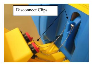
3. While holding the tray in this position making sure *not* to "pop" the red caps of the spray faces. Disconnect both "old style" beaded chain & clip assemblies from the red spray head caps, and the stainless steel split rings.
