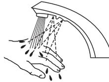
3. When hands are moved away from the OPTIMA® Sensor, the loss of reflected light initiates an electrical signal that deactivates the Solenoid Valve shutting off the water flow. The Circuit then automatically resets and is ready for the next user.
