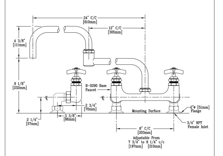
Note: Drill 1 1/4"ø [32mm] Holes on 8"c/c in Mounting Surface.
