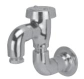
Engineering Specification: Zurn AquaSpec® Z800P0-SE Bedpan washer flanged wall supply with a vacuum breaker, a 1/2" female inlet and a 3/8" female outlet.
