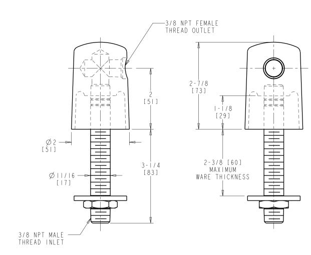
DIMENSIONS ARE IN INCHES AND [MILLIMETERS].
