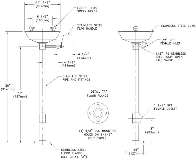
NOTE: EACH GS-PLUS SPRAY HEAD HAS A "FLIP-TOP" DUST COVER, INTERNAL FLOW CONTROL AND FILTER TO REMOVE IMPURITIES FROM THE WATER FLOW.
