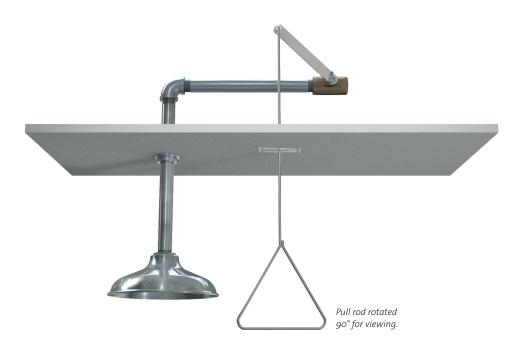
**APPLICATION:** Emergency shower for semi-concealed mounting in a finished ceiling. Unit is designed for installation in ceilings 8-10 feet above finished floor.
