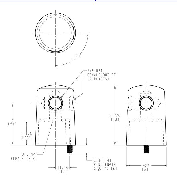
DIMENSIONS ARE IN INCHES AND [MILLIMETERS].
