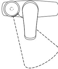
2. As the user's hands enter the beam's effective range, the beam is reflected back into the OPTIMA® Scanner Window and activates the solenoid valve allowing tempered water to flow from the faucet. Water will flow until the hands are removed or until the faucet reaches its automatic time out limit setting.
