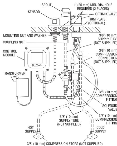
ETF-660 Faucet with BDM and BDT Variation Mixing Valves for Hot and Cold Water Supply (shown with 4" trim plate)
