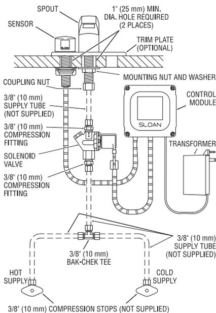
ETF-660 Faucet with ADM Variation Mixing Valve for Hot and Cold Water Supply (shown with 4" trim plate)
