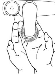
3. When hands are moved away from the "ON-Q®" OPTIMA® Sensor, the loss of reflected light initiates an electrical signal that deactivates the Solenoid Valve, shutting off the water flow. The Circuit then automatically resets and is ready for the next user.
