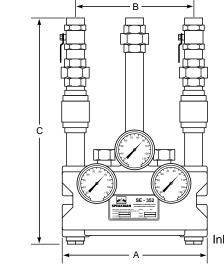
Inlet & Outlet 1<sup>1</sup>/<sub>4</sub>" N.P.T. Allow for 5" Depth
