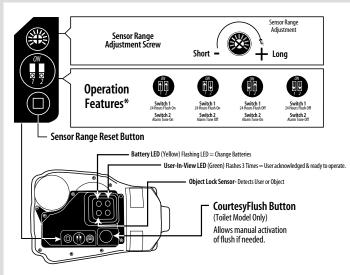
\*Trap Seal Protection (24hr flush): Ensures fixtures are flushed at least once every 24 hours. This feature prevents sewer gases escaping through open trap. This feature can be turned off by placing switch #1 in the down position. \*Battery Replacement Tone: Optional audio tone reinforces yellow LED (change batteries). This feature can be turned off by placing switch #2 in the down position.
