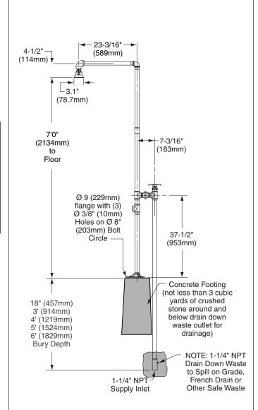
NOTE: All dimensions assume standard thread engagement. Variations in manufacturing allow for +/- 1/8" (3mm) per threaded joint. To find the tolerance of a dimension, add the number of thread joints in between a dimension and multiply it by 1/8" (3mm).
