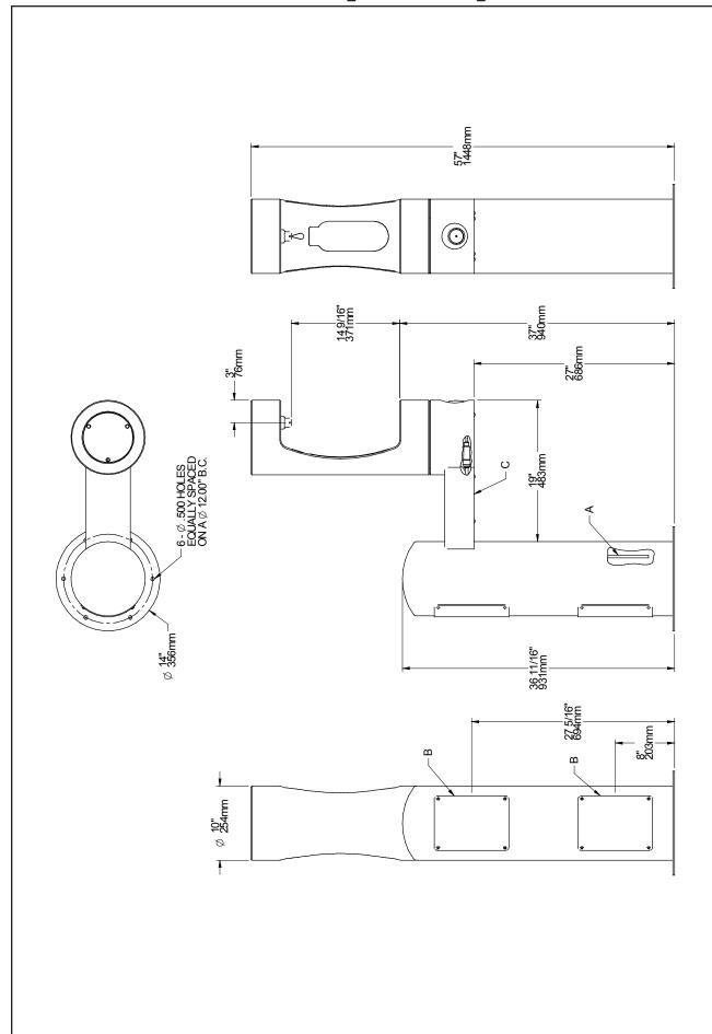
A = 3/8" O.D. UNPLATED COPPER TUBE CONNECT - SHUT OFF VALVE BY OTHERS B = ACCESS PANEL (8" X 10")
