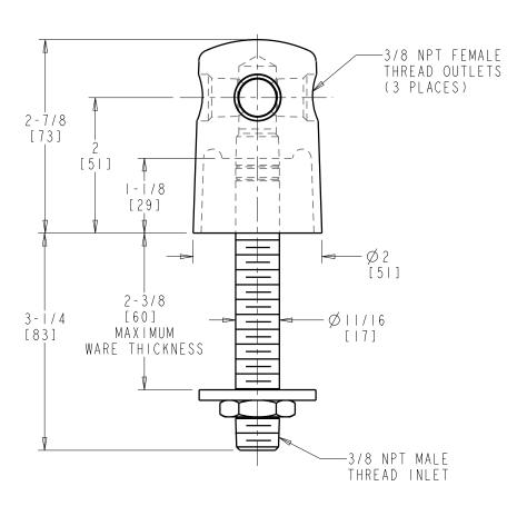
DIMENSIONS ARE IN INCHES AND [MILLIMETERS].
