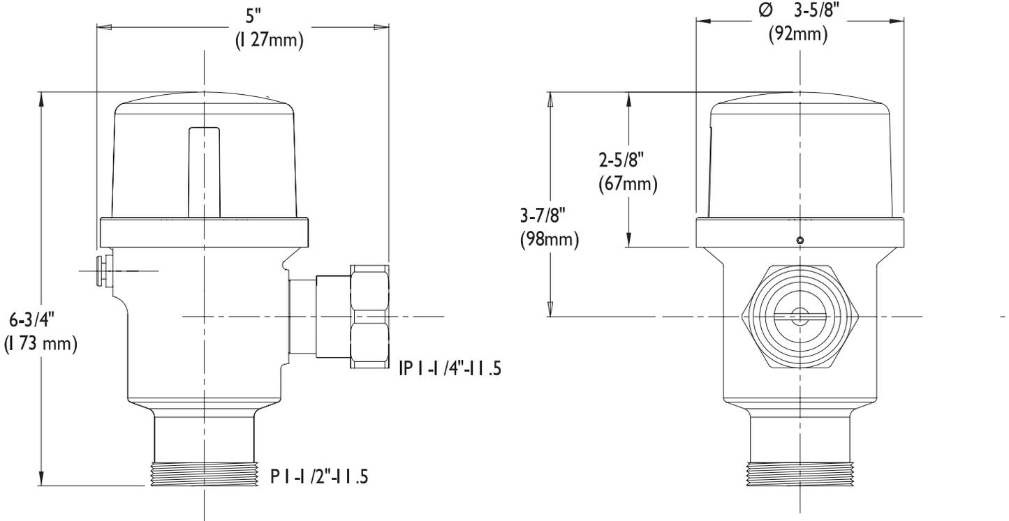
NOTE: All dimensions are in inches (millimeters) unless otherwise specified and are subject to change without notice. Unless otherwise specified, inlet is 1-1/4 NPSM female and outlet is 1-1/2 NPSM male.
