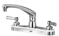
Polished chrome-plated 8" [203mm] brass deck faucet with an 8" [203mm] cast brass swing spout and quarter turn ceramic disc cartridge. Unit is furnished with a 2.2 GPM [8.3 L] pressure compensating aerator (complying with ANSI A112.18.1 Standard for flow), 2-1/2" [64mm] vandal-resistant color-coded metal lever handle, mounting hardware and 1/2" NPSM coupling nuts for standard lavatory riser.
