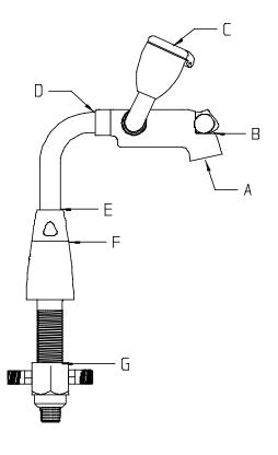
Step 4- Disconnect any hoses to the tee. Unscrew the tee and replace any necessary seals. Screw the tee back on tight and connect the hoses.
