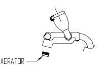
TENPERATURE LIMIT STOP RING ADJUSTMENT SCALE 3.000 MINIMUM MAXIMUM HOT HOT TEMPERATURE-LINIT STOP RING П POSITIO FLOW TEMP. L N @ 45 LIMIT IMIT PSI. MOVE DOWN FOR LESS FLOW 0% 0% 0 1 5% 0% FLOW LIMIT 2 12% 3% ADJUSTMENT 3 25% 10% 4 20% 5 30% 6 40%
