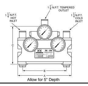
The Emergency Shower Mixing Valve shall employ two fully independent control mechanisms which split the flow in half, blend each half to the design temperature and then integrate each stream at the outlet. The valve shall control outlet temperature over a wide range of flow and shall be suitable for deluge shower or eyewash applications. The valve shall include three thermometers to measure the temperature of each stream and the merged flow. Temperature adjustment shall be vandal resistant.
