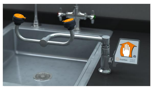
**APPLICATION:** All-stainless steel eyewash for mounting on counter next to sink. Spray heads swivel 90 degrees from storage to operational position. Unit is constructed entirely in stainless steel for corrosion resistance.
