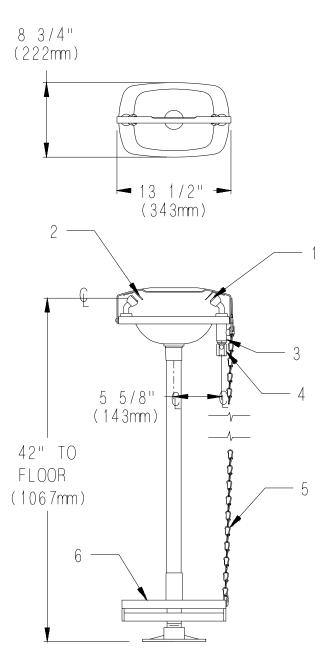
NOTE: This unit should be connected to an uninterrupted source of potable water, with a minimum flowing pressure of 30 PSI and a maximum static pressure of 125 PSI.
