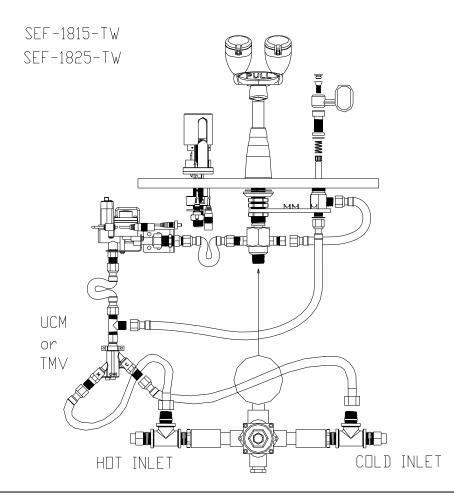
**SEF-1815-TW** -8" Sensorflow, eyewash faucet, UCM, MO, battery and Thermostatic Valve for Eyewash **SEF-1825-TW** -8" Sensorflow, eyewash faucet, UCM, MO, AC/DC and Thermostatic Valve for Eyewash
