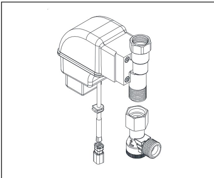
2.2. Open battery module using supplied Allen wrench and install supplied batteries in the electronics module.
