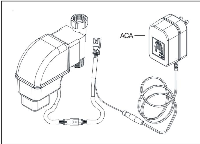
2.2b. Optional HW6 (Hardwired 6V) version: Connect supplied inline connector and hardwire adapter. When securing the CWB wires to the screw terminals on HW6 unit, the BLACK WITH DASHED MARKINGS should be connected to the Positive (+) terminal, and the SOLID BLACK wire should be connected to the Negative (-) terminal.
