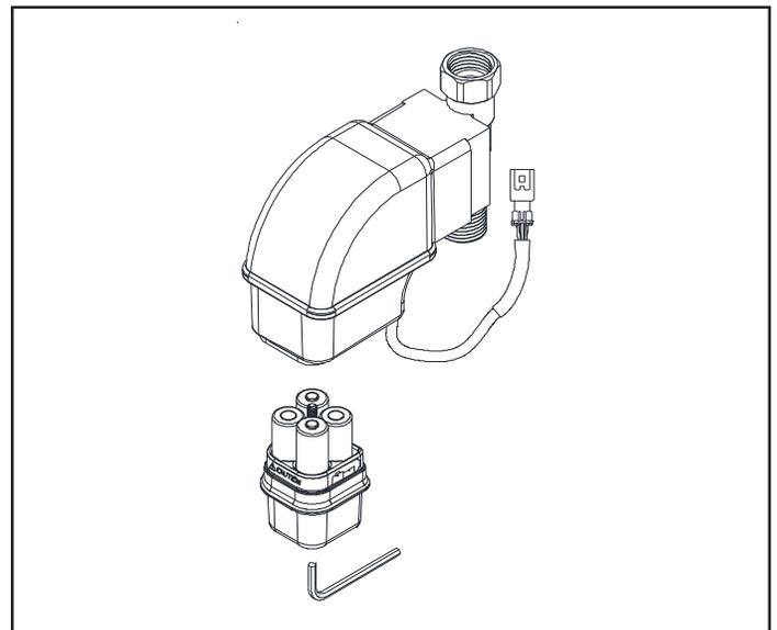
2.2a. Optional ACA version: Connect supplied inline connector and AC adapter.
