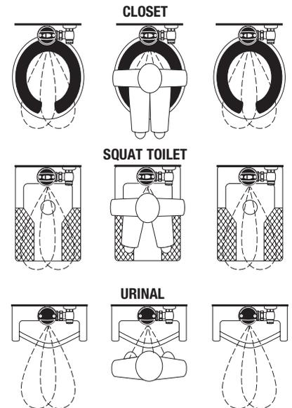
3. For a dual-flush model, once a user is detected, if the user leaves in 65 seconds or less, a reduced flush will automatically initiate. The circuit automatically resets and is ready for the next user. For a single-flush model, when the user steps away, this initiates a full flush. The circuit automatically resets and is ready for the next user.
