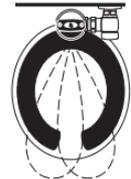
2. As the user enters the beam's effective range (22" to 42") the beam is reflected into the OPTIMA Plus Scanner Window and transformed into a low voltage electrical circuit. Once activated, the Output Circuit continues in a "hold" mode for as long as the user remains within the effective range of the Sensor.
