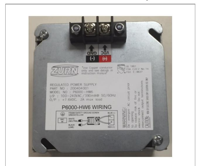
P6000-HW6 (7.6VDC) Hardwired Power Converter for Flush Valves and Faucets
