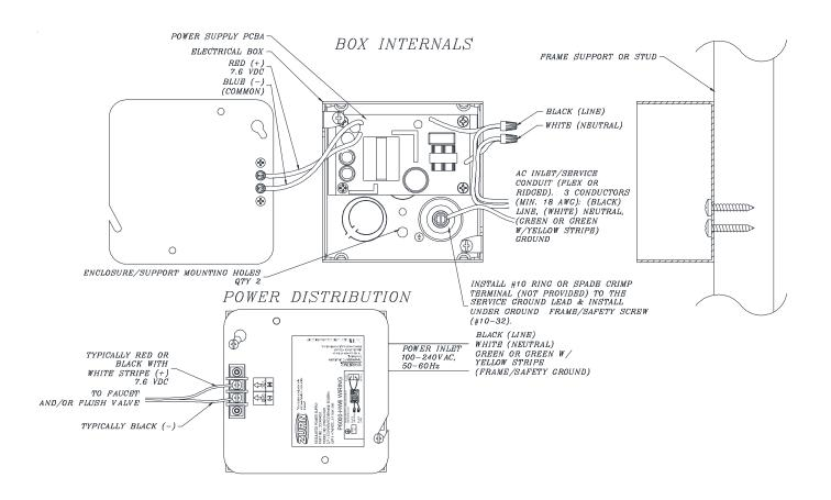
The internal (Line & Neutral) conductor terminations/connections, shall be implemented using UL approved screw terminals, wire nuts, insulated crimp splices, or soldered using hook & loop method with the solder joint(s) post insulated or as specified within the National Electrical Code (NEC) and/or superseding relevant local specified code(s).
