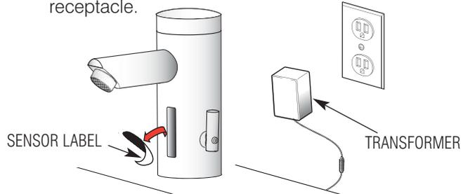
Electrical Connection for up to Six (6) Faucets Using One (1) Transformer
