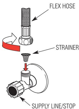
**B** Tighten the Flex Hose (with Strainer in place) securely to the Supply.
