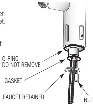
**B** Install Faucet with O-ring into the center hole in deck or lavatory — 1-3/16" (30 mm) min. hole required.
