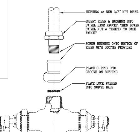
Product Description: Drawn: Checked Scale: WJS **MVW** 1:2 EASY INSTALL RETRO-FIT KIT: Approved Date: SWIVEL NUT, BUSHING, O-RING, & LOCK WASHER MVW 9/10/03
