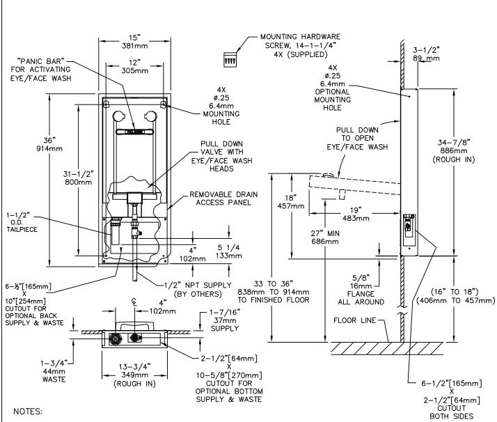
WHEN INSTALLING THIS UNIT, LOCAL, STATE OR FEDERAL CODES SHOULD BE ADHERED TO. WASTE CONNECTION MUST ADHERE TO LOCAL HEALTH AND PLUMBING CODES. FLOW RATE FOR EYE/FACE WASH IS 5 GPM AND EXCEEDS ANSI STANDARD Z358.1.
