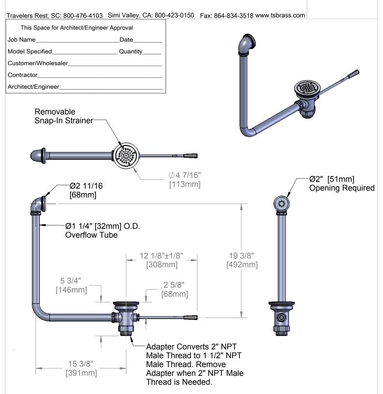
Waste Drain Valve w/ Lever Handle, 3 1/2" Sink Opening, 2" NPT Male Outlet, 1-1/2" NPT Male Adapter & Overflow Tube w/ Head Asm.
