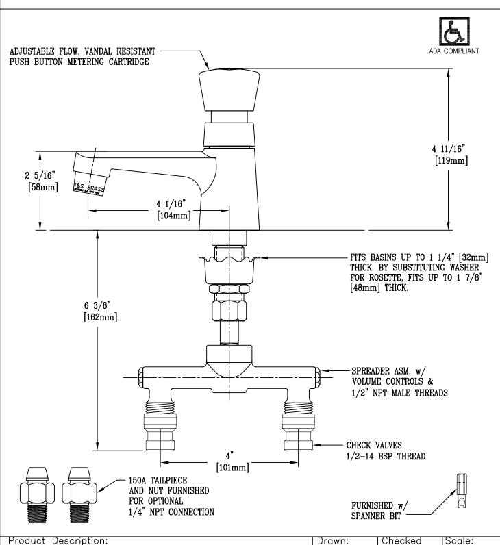
PUSH BUTTON METERING FCT. w/ AERATOR & BELOW COUNTER SPREADER ASSEMBLY & CHECK VALVES Drawn: Scale: **GEF** DHL 1:2 Date: Approved
