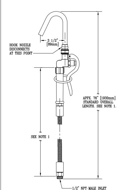
NOTE 1: STANDARD OVERALL LENGTH OF HOSE IS 76" FROM TOP OF GOOSENECK TO BOTTOM OF 1/2" NPT MALE INLET. MAY BE FURNISHED IN ANY LENGTH REQUIRED WHEN SPECIFIED.
