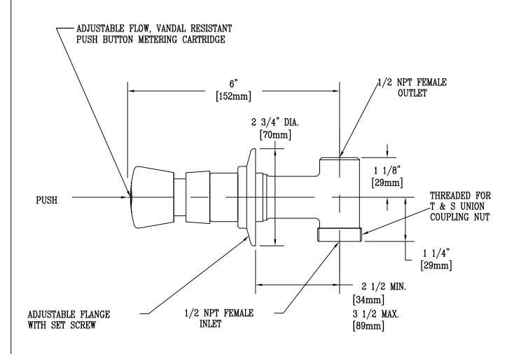
ADD - UCP SUFFIX FOR 1/2 IPS FEMALE UNION INLET ADD - UCT SUFFIX FOR 5/8 O.D. COPPER TUBING
