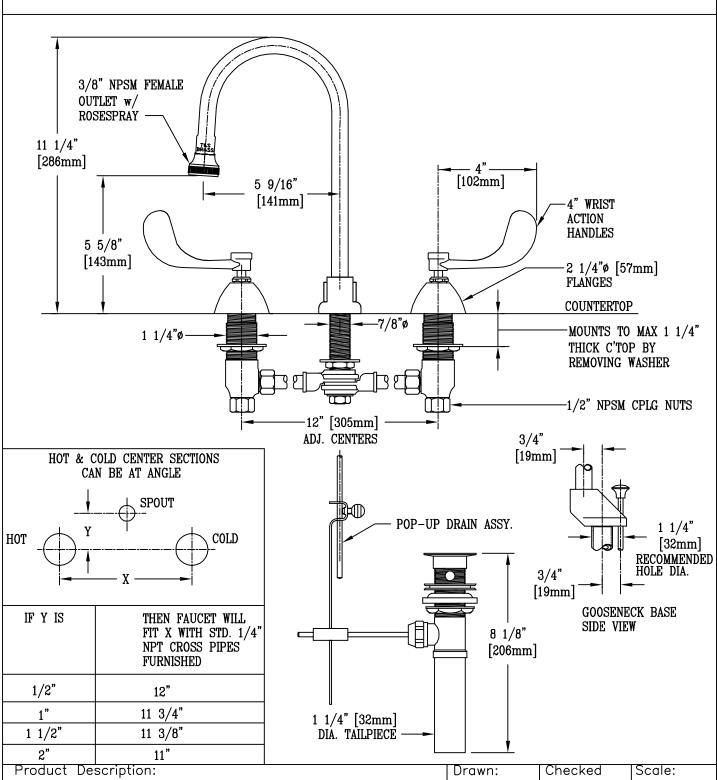
12" c/c DECK MOUNTED MIXING FAUCET w/ 4" WRIST ACTION HANDLES, ADJUSTABLE CENTERS, POP-UP DRAIN, & RIGID GOOSENECK WITH ROSESPRAY OUTLET
