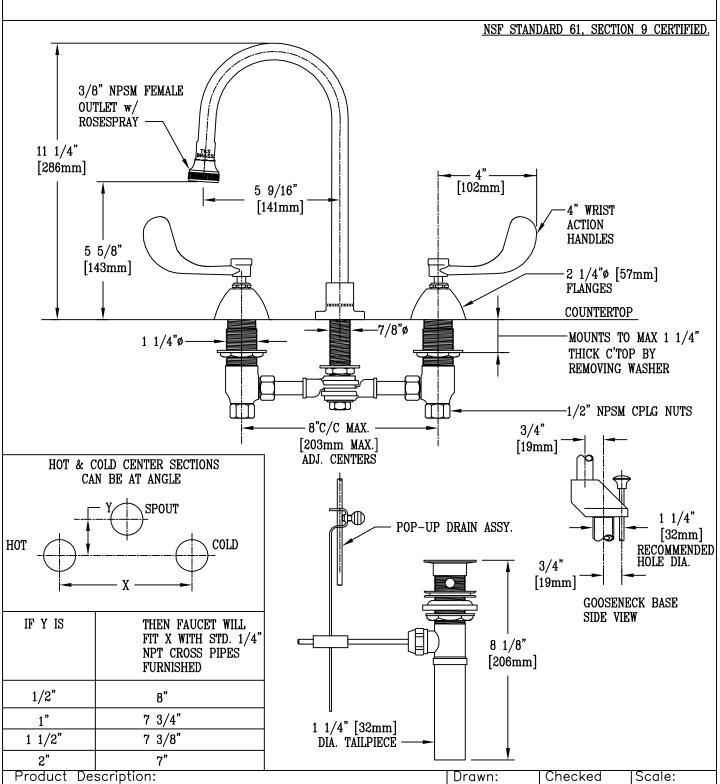
DECK MOUNTED MIXING FAUCET WITH 4" WRIST ACTION HANDLES, ADJUSTABLE CENTERS, POP-UP DRAIN, & RIGID GOOSENECK WITH ROSESPRAY OUTLET
